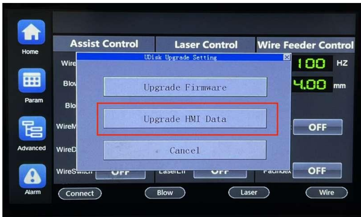
Figure 5-1: Touch screen program upgrade
