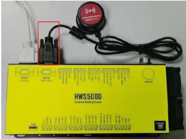
Figure 7-6 (Wireless receiving module installation)
