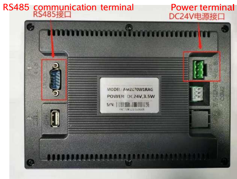
Figure 6-1: Touch screen wiring terminal
